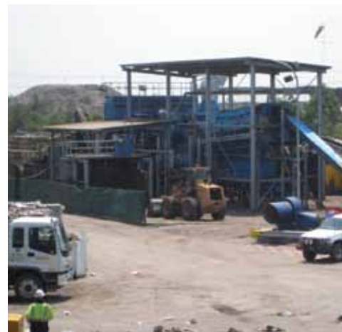
The Global Renewables compost is screened multiple times to try to remove remaining plastic and glass.
