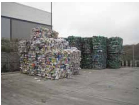
Bales of PET and HDPE plastics arrive at Closed Loop Recycling from the Veolia-operated MRF.
