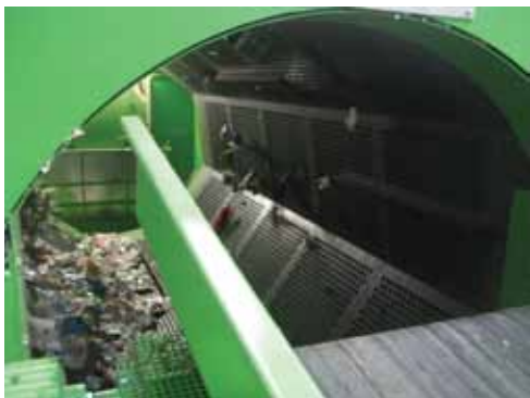
Plastic bottles are sent through a trommel for the initial sort at CLR.
