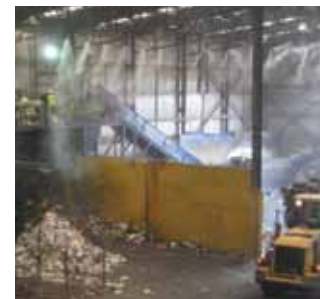
Workers at Global Renewables hand pick recyclables from the residual municipal solid waste stream. Misting is used to prevent dust.
