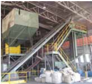
Materials are sorted again through a mini-MRF by the supercollector, weighed, and baled.
