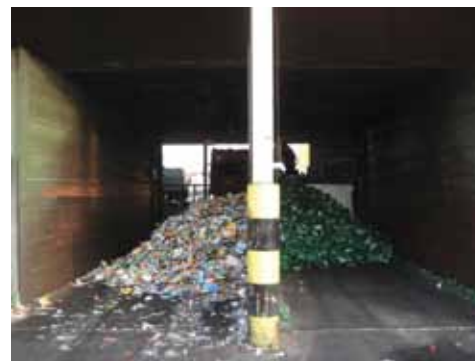
Separated materials are collected in bunkers before being baled (drinks cartons on left, green PET bottles on right).
