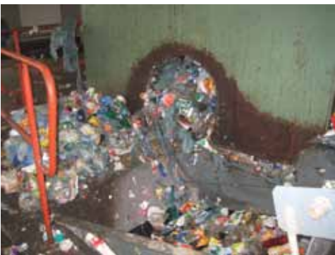
Full bags are broken by a toothed screw, allowing bags and PMD materials to fall to a conveyor belt for sorting.
