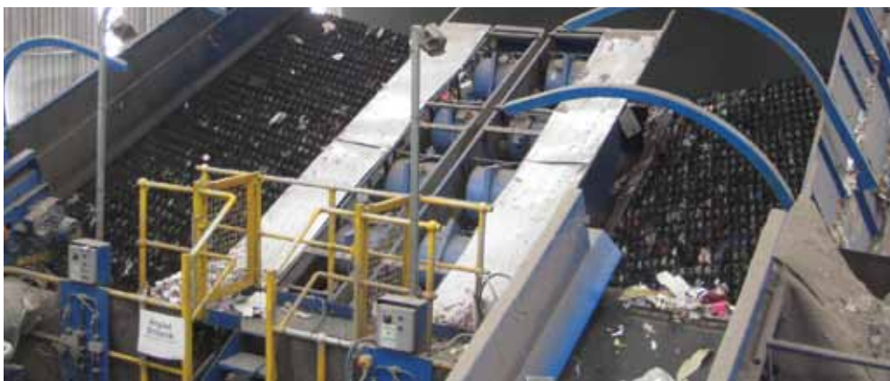
The slanted (or angled) screens separate flat paper (stays on the outer edge of the screen) from three-dimensional containers (roll down the slope).
