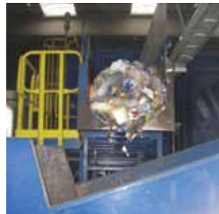
A screw opens the bags, allowing the contents to be sorted.
