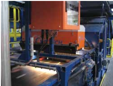
An optical Ti-tech sorter separating plastics at high speed.
