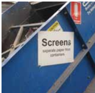
The screen separates large paper items from smaller paper items and containers.
