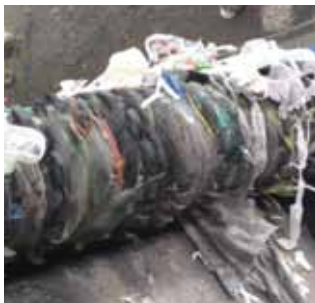
Plastic film, netting, and other contaminants bind the screening equipment and cause frequent work stoppages for cleaning.
