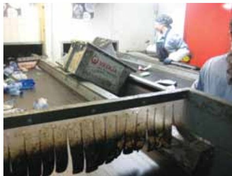
Hand sorting is used for quality control. A worker ensures only drinks cartons are on the conveyor belt.
