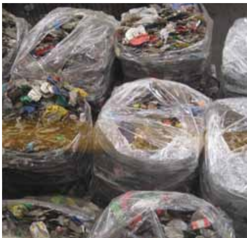
Containers of recyclables hand-picked from the residual municipal solid waste stream. The materials are quite dirty.
