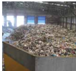
Residual municipal solid waste is brought to the Global Renewables' receiving area.
