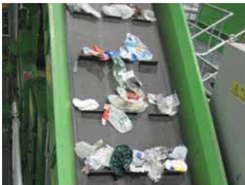
The mixed plastic bottles are sent through a series of sorting technologies to remove aluminum and steel, and then to an optical sorting machine to be separated by polymer type.
