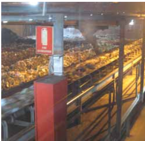
Everything not sorted out as recyclable goes to composting. The waste, which is approximately 40% plastic, is composted on conveyor belts inside a building with negative air pressure to reduce odor outdoors.
