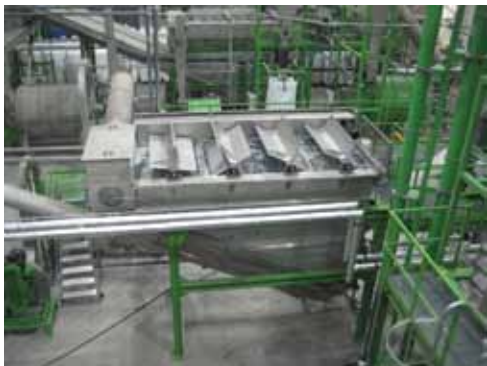
The plastic flakes are washed and sent through a float-sink operation.
