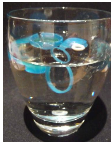
b) Cap and rubber seal float while silicone valve sinks
