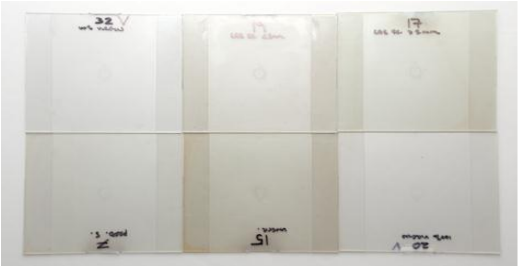
Figure 18: Example of the type of discolouration occurring in moulded plaques when virgin PET is mixed with PET and other 13% of plastic fines. (The top left and bottom right plaque are virgin control samples for comparison)
