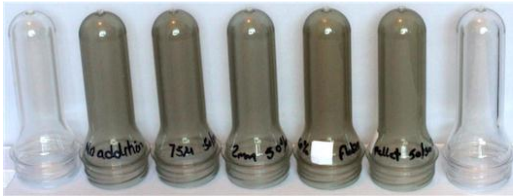
Figure 21: rPET materials from different recyclers display different colours. Outer preforms are virgin preforms for comparison, material for the three discoloured preforms on the left are from Recycler A and next two are from Recycler B.
