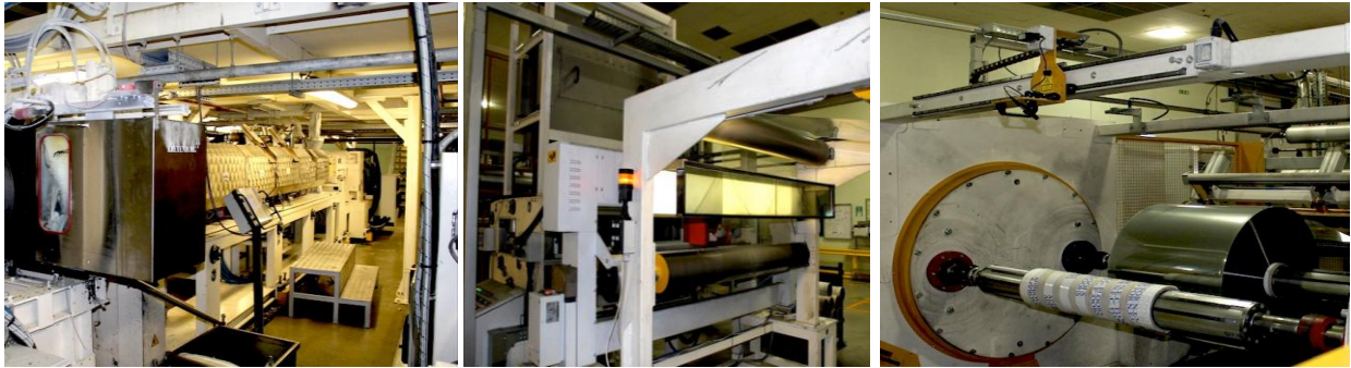
Figure 27: Sheet extrusion trial using screened flakes (Courtesy of Anson Packaging).
