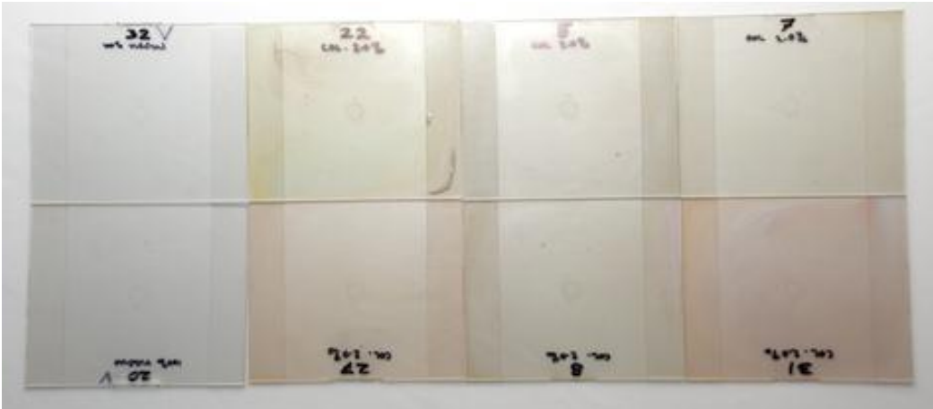
Figure 14: Example of the type of discolouration occurring in moulded plaques when virgin PET is mixed with 1.3% of mixed coloured PET particles. (The top left and bottom left plaques are virgin control samples for comparison)
