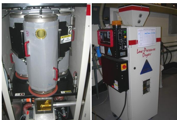
Figure 8: An example of the Maguire low-pressure dryer used to dry the virgin PET at 150°C for 30-35 minutes.
