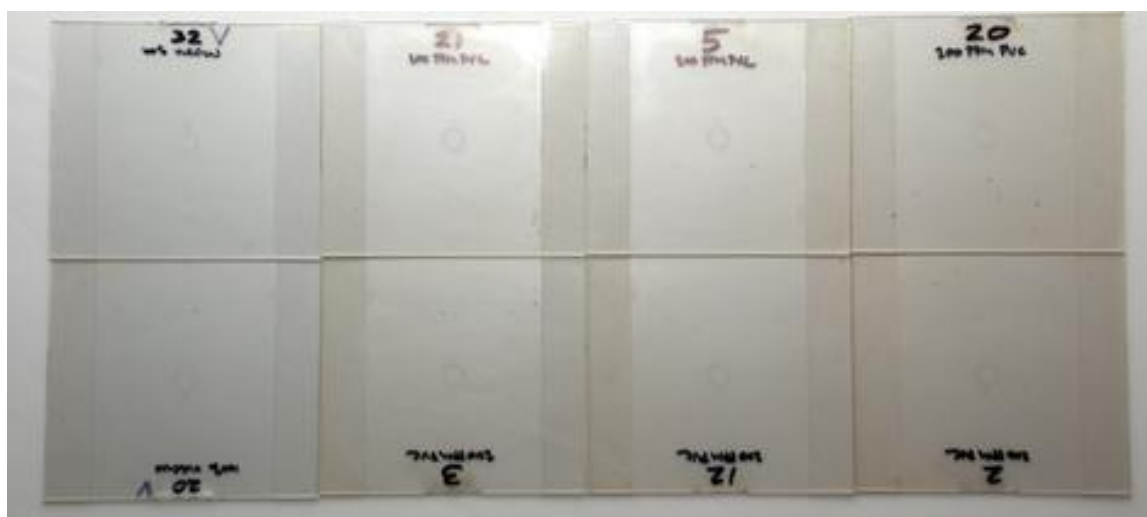
Figure 11: Example of the type of discolouration occurring in moulded plaques when virgin PET is mixed with 200ppm of PVC particles. (The top left and bottom left plaques are virgin PET control samples for comparison and all others are plaques moulded with 200ppm PVC)
