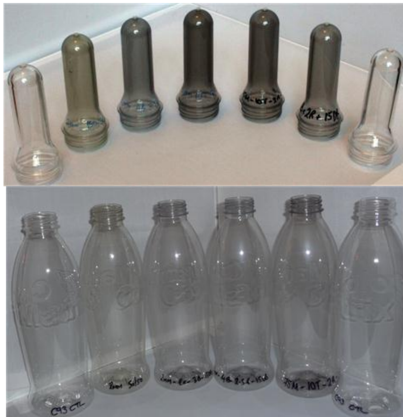
Figure 22: Preforms and bottles made with 50% rPET from Recycler A and mixed with a series of different levels of toners and optical brighteners.
