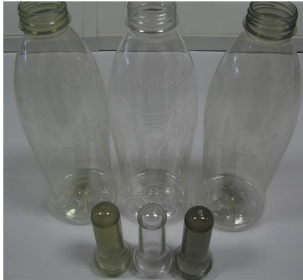
Figure 23: Preforms and bottles made with 50% rPET from Recycler B and a series of toners and optical brighteners.
