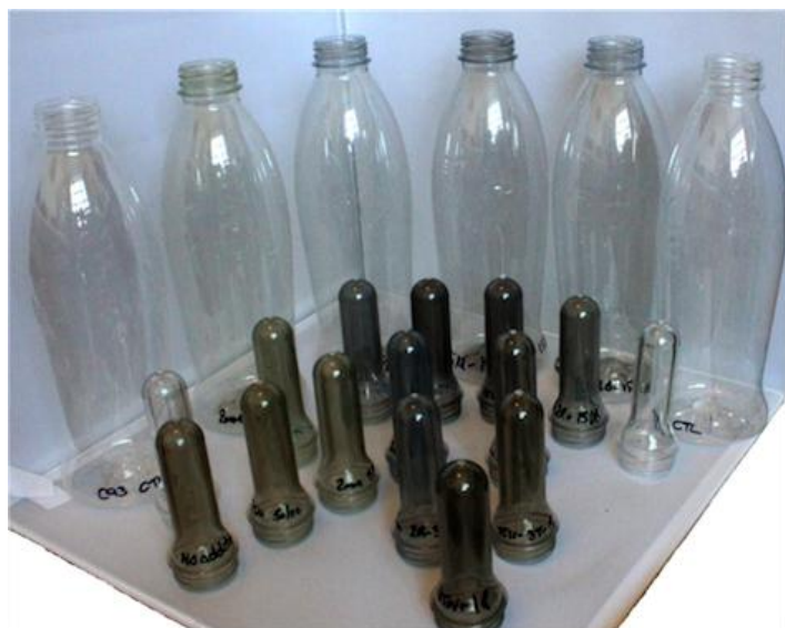
Figure 20: Example of colours of preforms and bottles made with 50% rPET and additions of toners and optical brighteners using flake from UK recycler A.
