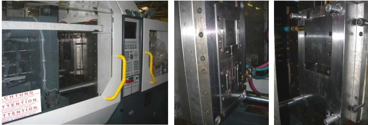
a) Demag ET 150 injection moulder fitted with a general purpose 25mm screw
