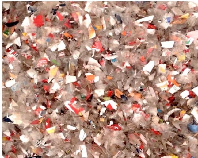
Figure 6: Example of granulated flakes with labels prior to several air classification and washing steps.
