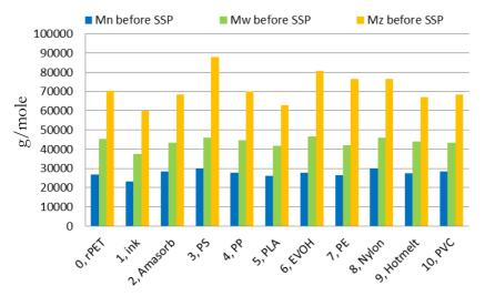
Figure 18: The three types of average molecular weights for the PET samples prior to SSP treatment.
