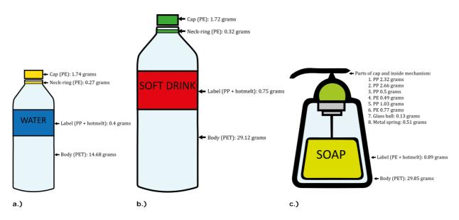
Figure 7: The material composition of some typical PET bottles and flask. a.) typical transparent PET bottle 0.5 L. b.) typical transparent PET bottle 1.5 L c.) typical non-food soap flask with pump mechanism
