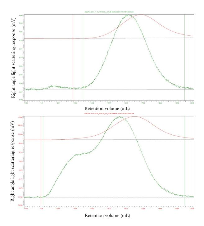
Figure 20: Gel-partitioning chromatogram for normal rPET (above) and rPET to which EVOH is added (below). In GPC's the largest masses run first of the column and the smallest masses as last. Hence the broad shoulder on the left side indicates the presence of molecules with a high molar mass. Red line = refractive index response, [mV] Green line = Right angle light scattering response, [mV]
