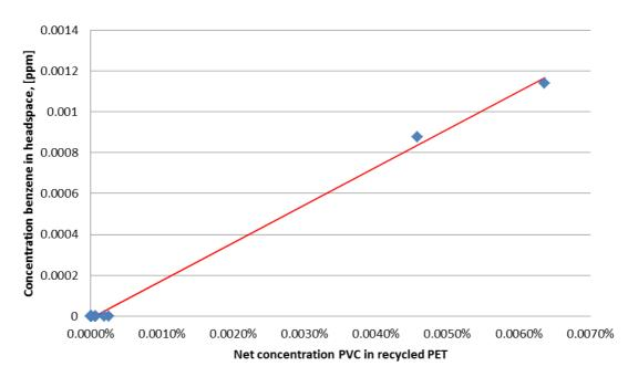
Figure 38: The correlation found between the measured benzene emission values in the headspace after SSP treatment in the samples of task 3 and the estimated concentration of PVC in these samples.
