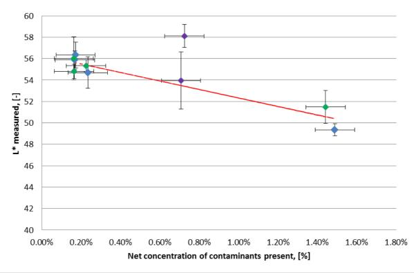
Figure 37: The correlation found between the measured L\* lightness value for the sample of task 3 and the total concentration of contaminants estimated to be present in these samples. The colours indicate the collection systems: purple for deposit-refund systems, green for separate collection systems and blue for mechanical recovery systems.
