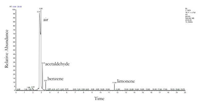
Figure 4: Volatile components as measured using head space gas chromatography. (Acetaldehyde at 3.14 min, benzene at 3.51 min and limonene at 11.64 min)
