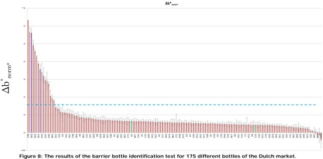
Figure 8: The results of the barrier bottle identification test for 175 different bottles of the Dutch market. Displayed are the normalised differences in b\* colour value. The purple bars are for known barrier bottles, the green bars for known non-barrier bottles. The blue dashed line is the threshold value of 1.6.
