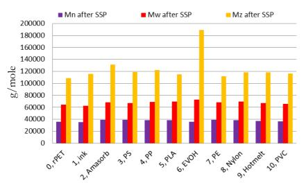
Figure 19: The three types of average molecular weights for the PET samples after SSP treatment.
