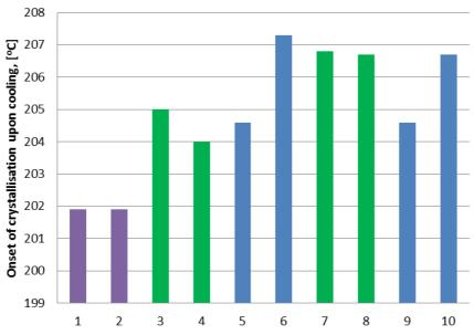
Figure 33: Onset of crystallisation derived from the cooling run [°C]. The colours indicate the collection systems: purple for deposit-refund systems, green for separate collection systems and blue for mechanical recovery systems.
