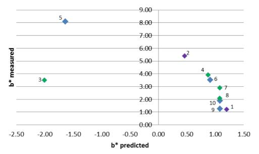
Figure 35: example of modelling b\* with the derived property parameters and the concentrations of contaminants present in the samples of task 3 after recycling. The colours indicate the collection systems: purple for deposit-refund systems, green for separate collection systems and blue for mechanical recovery systems.
