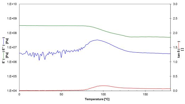
Figure 23: Typical DMTA thermogram of semi-crystalline PET.
