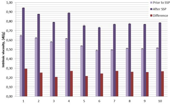
Figure 30: The intrinsic viscosities of the ten combinations of feedstock and process before and after the SSP treatment.
