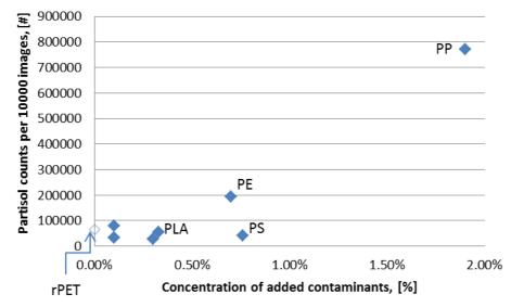
Figure 15: Relationship between the concentration of added contaminants and Particle count.
