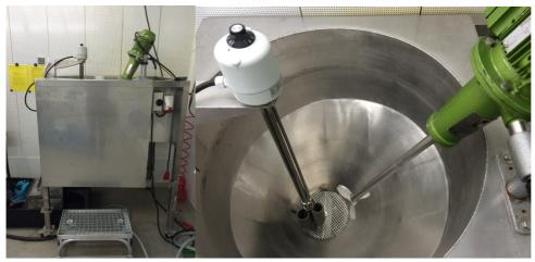
Washing mill (outside and inside), including heater. Heater is removed before washing process.
