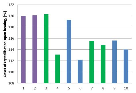
Figure 34: Onset of crystallisation upon heating the rPET, derived from the first heating run [°C]. The colours indicate the collection systems: purple for deposit-refund systems, green for separate collection systems and blue for mechanical recovery systems.
