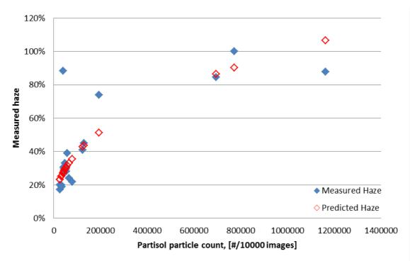
Figure 39: correlation between the measured haze values for the samples of task 2 and 3 and the measured partisol counts for the same samples.
