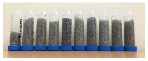
Figure 14: Samples of the recycled PET granulates. Variations in the greyish colour caused by contaminants. From left to right: 0 rPET, 1 ink, 2 Amosorb, 3 PS, 4 PP, 5 PLA, 6 EVOH, 7 PE, 8 Nylon, 9 Hotmelt, 10 PVC.
