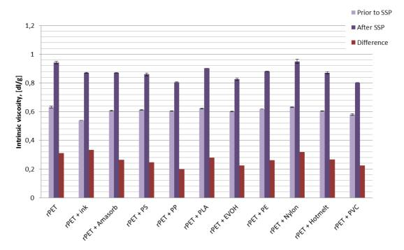
Figure 17: The Intrinsic viscosities of the rPET granulates prior and after SSP [dl/g].
