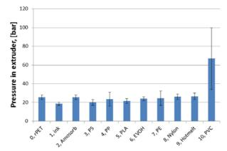
Figure 13: The pressure in the extruder during processing the samples for task 2 [bar].
